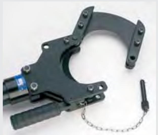
Opening head, to allow cutting of running cables
